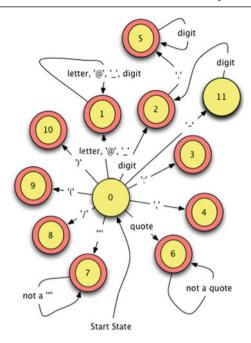
Fig. 4.29 The JCoCo scanner FSM
