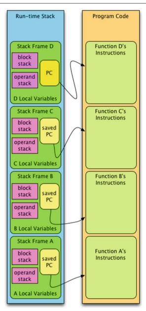
Fig. 3.1 The JCoCo virtual machine
