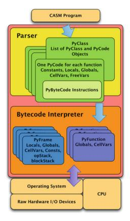
Fig. 4.2 The JCoCo virtual machine
