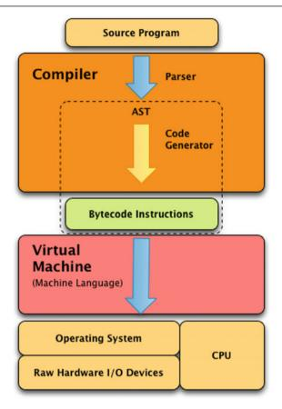
Fig. 1.14 Virtual machine implementation
